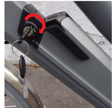
To remove the battery, turn the key to the right
